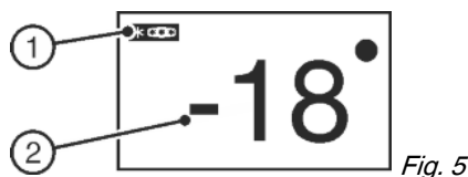
Fig. 5 (1) Freezer compartment symbol (2) Freezer compartment temperature display
