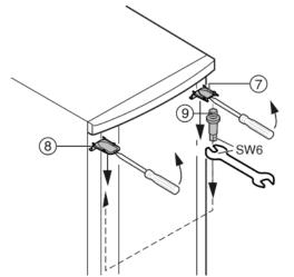
▶ At the top, use a screwdriver to unclip cover Fig. 6 (7) and cover Fig. 6 (8) at the front, and remove by pulling out and down.
