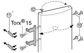
▶ Lift the stopper Fig. 7 (12) out of the door bearing bush and transfer it.
