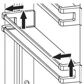
By shifting the **bottle holder** you can protect the bottles from falling over when opening or closing the door.
