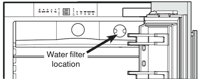
Replace the filter when the waterdrop symbol appears in the temperature display.
