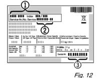
Notify the customer service, specifying the fault, appliance designation Fig. 12 (1), service No. Fig. 12 (2) and serial No. Fig. 12 (3).
