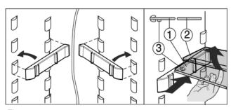
Fig. 4The glass plate (1) with pull-out stops must be at the front so that the stops (3) face downwards.
