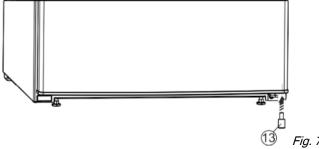
▶ Insert the spacer Fig. 7 (13) back under the right-hand side of the door, as it is important for the stability of the appliance.
