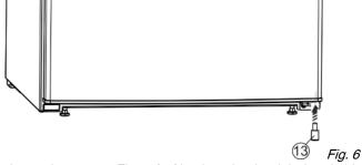
▶ Insert the spacer Fig. 6 (13) back under the right-hand side of the door, as it is important for the stability of the appliance.
