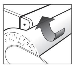
■ If you now lift the finger guard, the roller stops rotating and the heater plate rises up.
