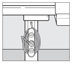
Unwind the cable. Do not insert the plug into the electrical socket yet.
