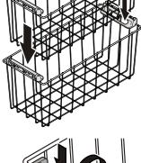
Press the handle downwards, lift and tilt inwards.
