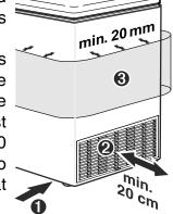
• Standard EN 378 specifies that the room in which you install your appliance must have a volume of 1 m³ per 8 g of R 600a refrigerant used in the appliance, so as to avoid the formation of inflammable gas/air mixtures in the room where the appliance is located in the event of a leak in the refrigerant circuit. The quantity of refrigerant used in your appliance is indicated on the type plate.
