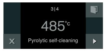
A signal sounds once the pyrolytic self-cleaning function has ended. A message appears in the display. Once the appliance has cooled down, wipe out the ash that has been left behind in the cooking compartment with a damp cloth.
