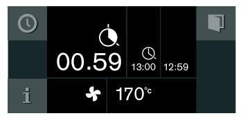
The appliance switches off after the cooking time has elapsed. The symbol flashes and a signal sounds. The signal stops when you touch the  $\checkmark$  symbol, open the appliance door, or switch the function selector to **0**.
