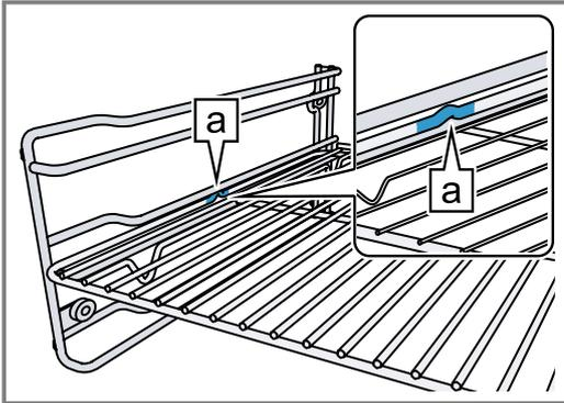
2. Ensure that the safety bracket on the wire rack is located at the rear and is facing upwards.
