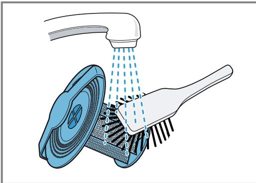
4. If it is very dirty, rinse out the drain filter under running water or clean it in the dishwasher.
