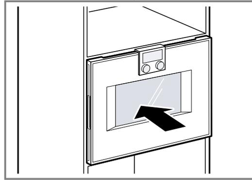
5. Centre the appliance. There must be an air gap of at least 5 mm between the appliance and the adjacent unit fronts.
