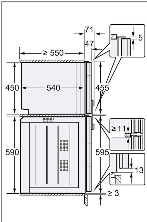
3. If there is no intermediate floor above the appliance, secure the appliance against tipping in the unit. Secure 2 commercially available brackets on both sides in the unit at a depth of 450 mm, 5 mm above the height of the appliance.
