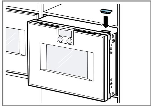
8. Slide the appliance into the built-in recess.
