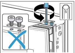
4. Adjust the appliance door using the side screw; to do this, open the appliance door and then close it again if necessary.
