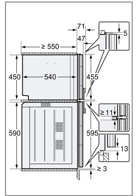
**3.** If there is no intermediate floor above the appliance, secure the appliance against tipping in the unit. Secure 2 commercially available brackets on both sides in the unit at a depth of 450 mm, 5 mm above the height of the appliance.
