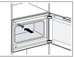
**9.** Remove the red plastic transport lock from the upper door catch.
