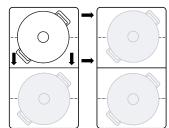
The cookware is detected and the previously selected power level flashes on the display for the new cooking zone.
